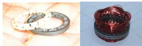
**Figure 6:** The stator coil of the resolver consists of the lamination (metal, left) wound with wire in a variable pattern (right). The white ring on the left is an end insulator.
